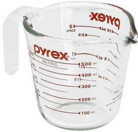
b. **Measure the volume** of the rock. Put the rock in a household measuring cup or bowl with measuring marks. Make sure the cup is bigger than the rock. Fill the cup with water. Measure the level in milliliters (mL). Take the rock out of the cup. Measure the water level again in milliliters (mL). Subtract the second number from the first to get the rock volume. (1 fl oz = 30 mL; 1 cup = 237 mL)
